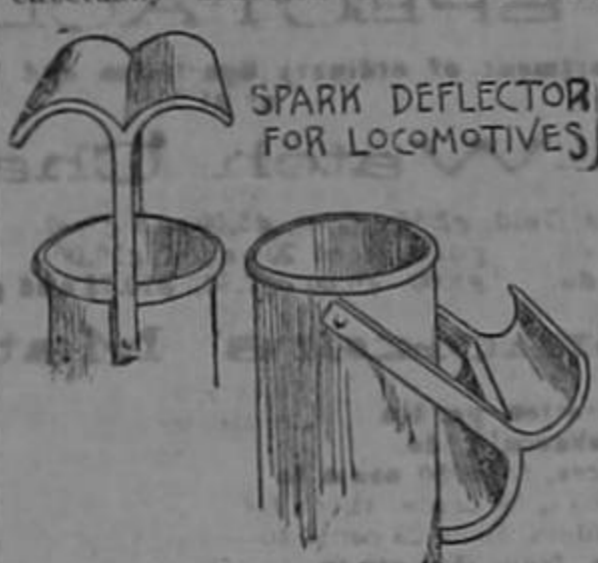
SPARK DEFLECTOR FOR LOCOMOTIVES.
